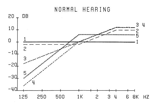
Figure 4. Schematic frequency responses for the five systems including differences in comfortable listening levels used in the experiment.
