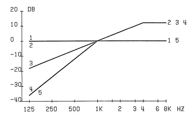
Figure 1. Schematic electrical responses of the five filters.
